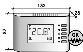
CR25 • FAN: MOT_AC~230V • Valvole-Valves: ON/OFF, PWM, 3-Point
